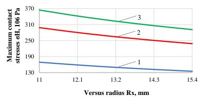
Fig. 4. Graphs of changes in the maximum contact stresses  $\sigma_H$  versus the radius  $R_x$ : 1 - F = 100 N; 2 - F = 550 N; 3 - F = 1000 N
