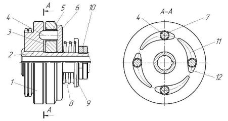
Fig. 1. Design diagram of the safety clutch: 1 – driving semi-clutch; 2 – hub; 3 – driven semi-clutch; 4 – cylindrical pins;5 – antifriction bushings; 6 – pressure disk; 7 – holes; 8 – spring; 9 – washer; 10 – nut; 11 – circular working grooves; 12 – circular reverse grooves
