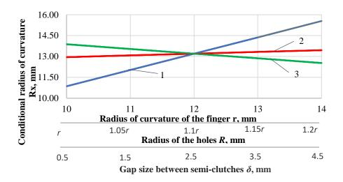
Fig. 3. Graphs of changes in the conditional radius  $R_x$  of curvature depending on: 1 – radius of urvature of the finger r; 2 – radius of the holes R; 3 – gap size  $\delta$  between semi-clutches
