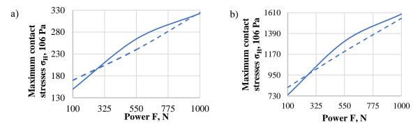
Fig. 7. Graph of changes in contact stresses depending on the force of the contact elements of engagements: a – pin-hole; b – pin-groove
