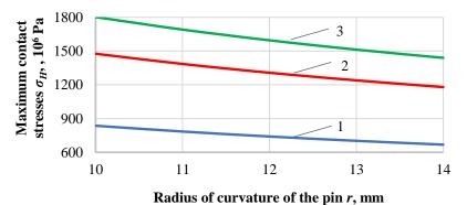
Fig. 5. Graphs of changes in maximum contact stresses  $\sigma_H$  versus the radius *r* of curvature of the pin: 1 - F = 100 N; 2 - F = 550 N; 3 - F = 1000 N
