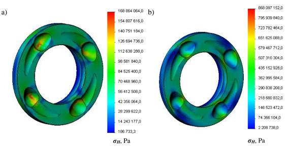
Fig. 6. Diagrams of distribution of the contact stresses in the engagements of the safety clutch: a – pin-hole; b – pin-groove
