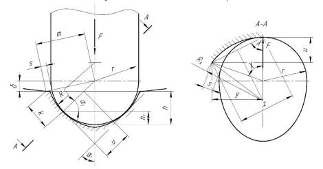
Fig. 2. Calculation scheme for determining the radius, describing the radius  $R_x$  of the hole in the plane of action of the force F
